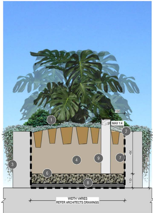
TYPICAL 600mm DEEP PLANTER SCALE 1:10
