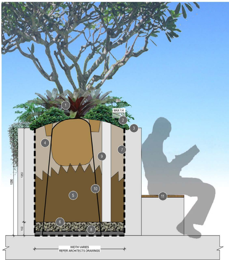
TYPICAL 1200mm DEEP PLANTER WITH SEATING SCALE 1:10
